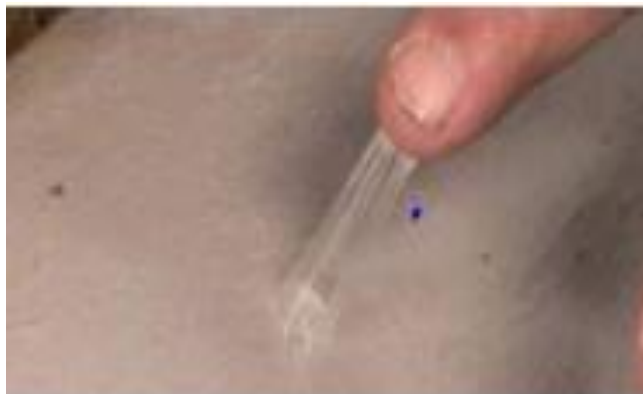
Figure 27 – Solvent Based Adhesive “Producing Strings”
